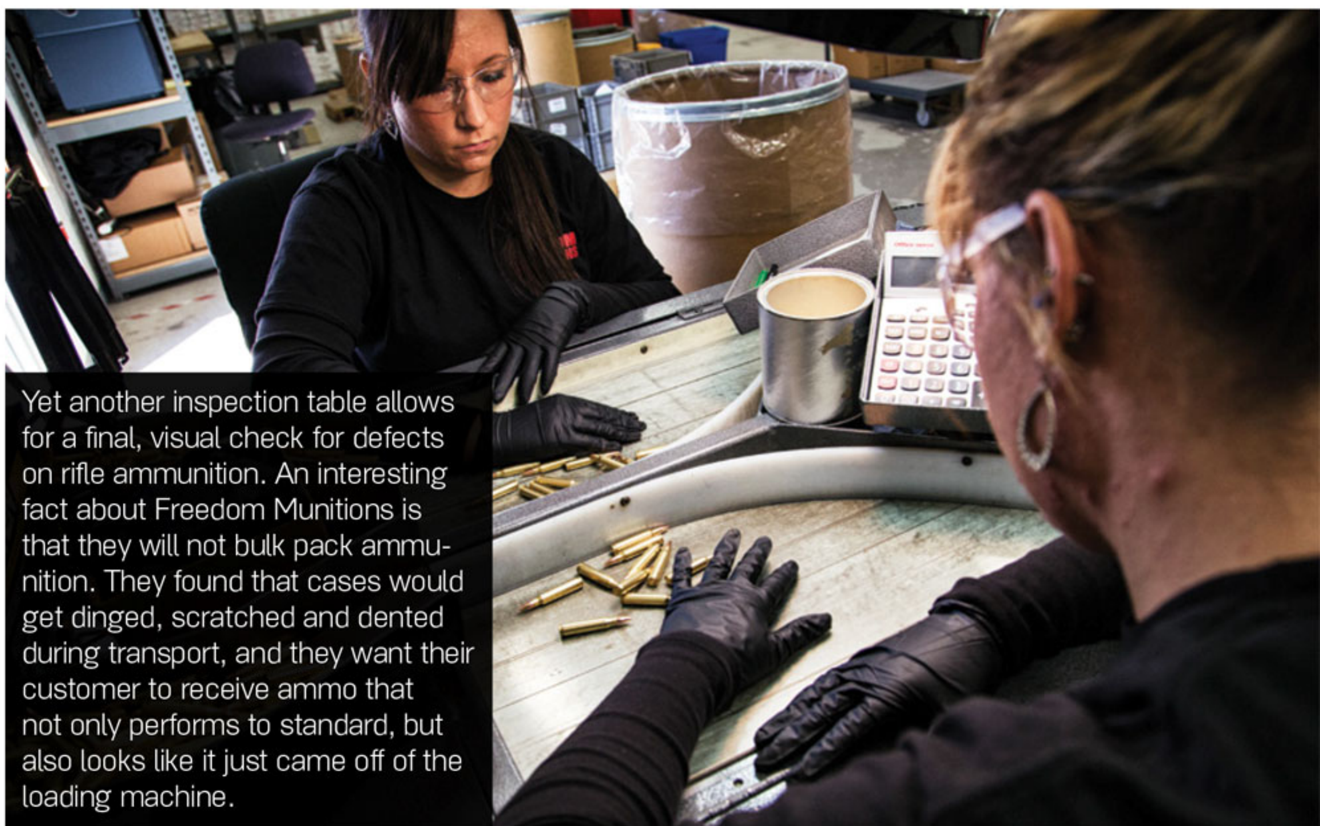
After being run through a mechanical sorting operation, each case is run across an inspection table like this one. Two seats at each table let the dedicated employees sort between the similar cases by hand.
