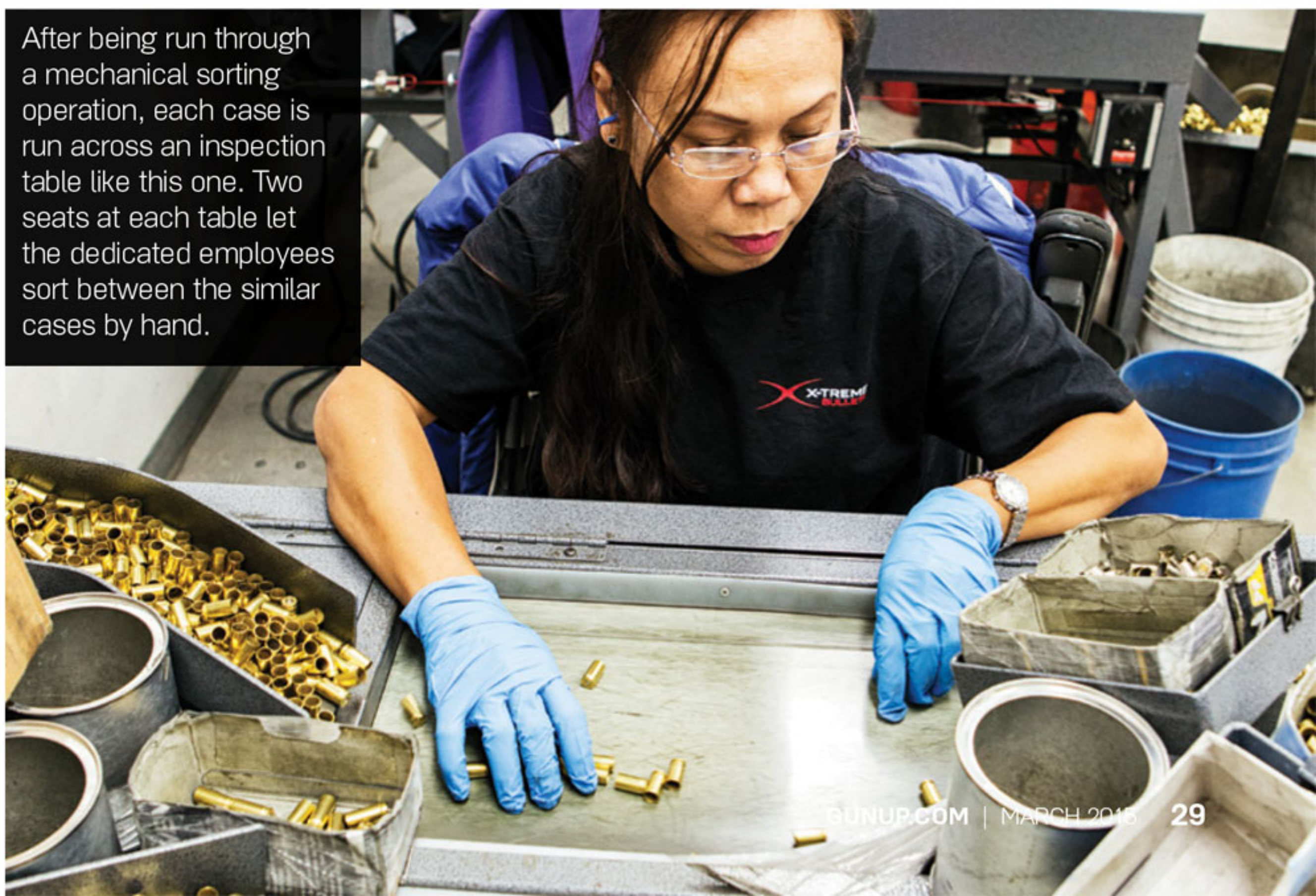
Yet another inspection table allows for a final, visual check for defects on rifle ammunition. An interesting fact about Freedom Munitions is that they will not bulk pack ammunition. They found that cases would get dinged, scratched and dented during transport, and they want their customer to receive ammo that not only performs to standard, but also looks like it just came off of the loading machine.
